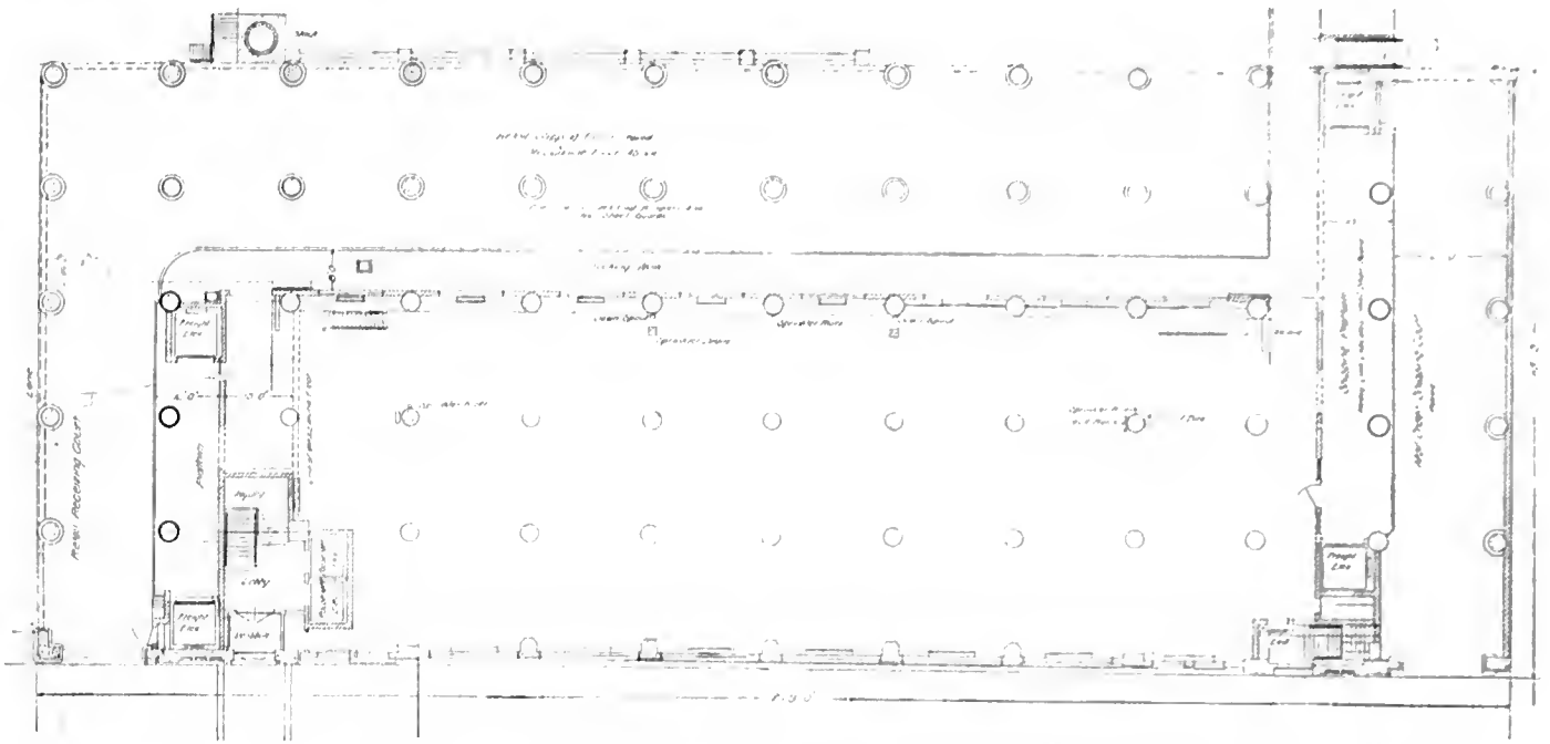
Fig. 2.—Ground Floor Plan of the New Robt. Simpson Mail Order Building Showing Arrangement of Foundation Piers, and Shipping Courts.
